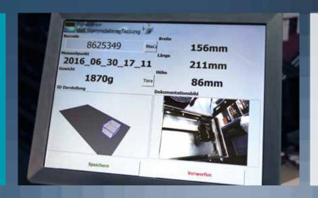
"The VLG static dimensioner combines fast measurement, independently of a specific person, with weight capture in a single step.
